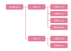
Linksper is implemented with an IFC-based model consisting of a main Site/Building/Floor/Space/Equipment tree and the ability to describe zones. The model is custom built for the site.
